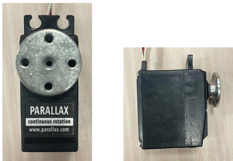
Figure 5b: Servo motor with horn attached front view (left) and side view (right)
