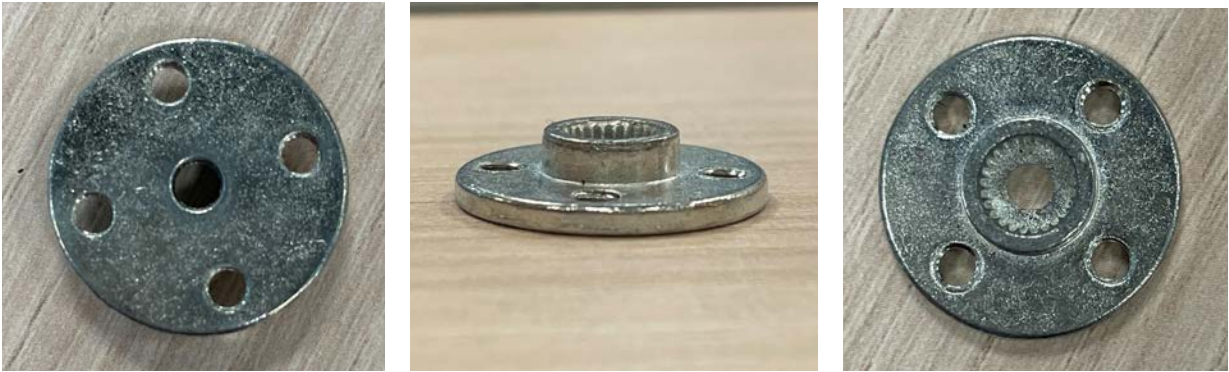
Figure 5d: Servo motor horn front view (left), side view (center), and back view (right)
